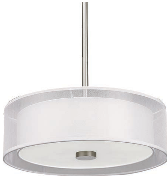
243-722/ST/BCH Brushed Chrome 3 x 60W med. base fabric shade# 065122/P bottom gl# 035122 ht 6" dia 22" rods 2 x 6" & 2 x 12"
