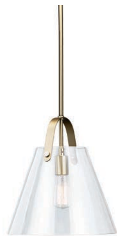
237-012/SG/CL Soft Gold 1x 100W med. base gl# 035371 clear ht 13 3/4" dia 12 3/4" rods 2x6" & 2x12"
