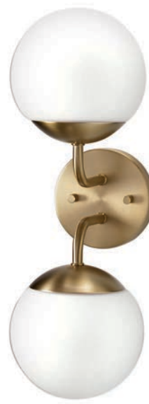
788-002/SG/OP Soft Gold 2x 60W med. base gl# 030880 opal ht 17" dia 6" extension 7 1/4"
